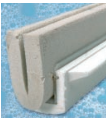
The sponge rubber is wearing, becoming softer and starting to become porous. The product must be replaced when this occurs.
